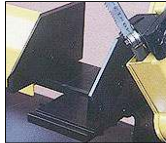
Adjustable blade guides allow the user to true up the vertical direction of blade, even when blade is worn.
